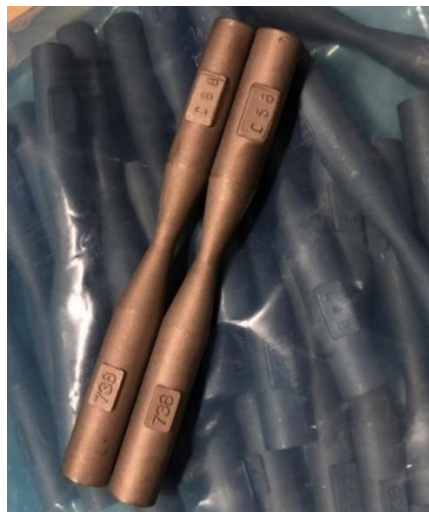
Figure 2.2: Blank sample produced by vacuum investment casting
