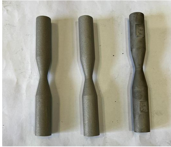
Figure 2.4: Sample surfaces after the aluminum oxide sandblasting
